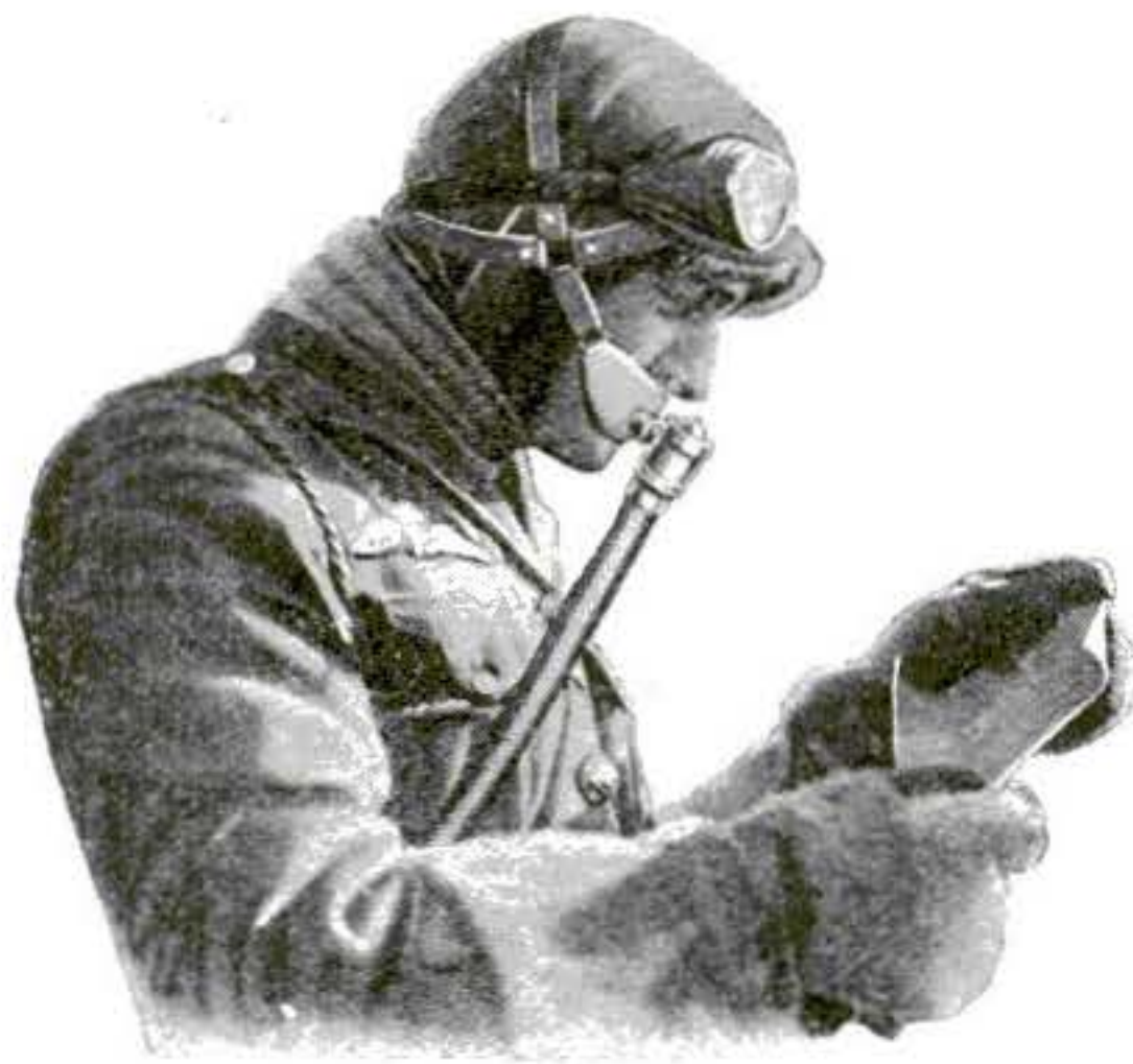
This simple-looking apparatus makes the unbreathable air of a 20,000-foot altitude possible to inhale. The tube is attached to a bottle containing oxygen
