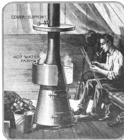
Just slip the ring-shaped vessel over the camp-stove when you want hot water
