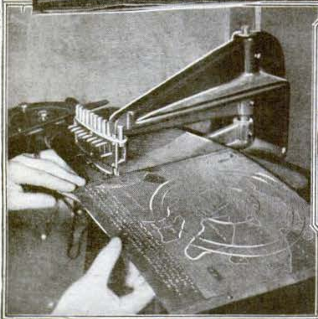
The machine that makes the forms from which maps are printed has eight dies, which, used singly or in combination, produce almost any sort of embossed lines. The map is that of the north polar region
