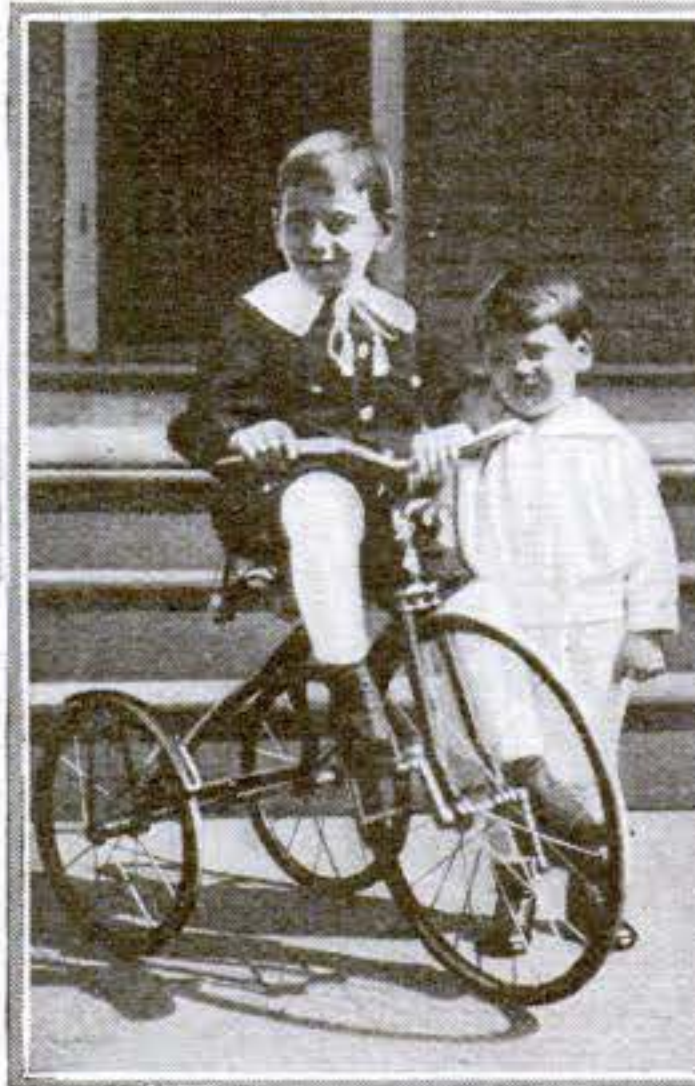
The new velocipede is strong and like a bicycle in design, with steel spokes and ball bearings
