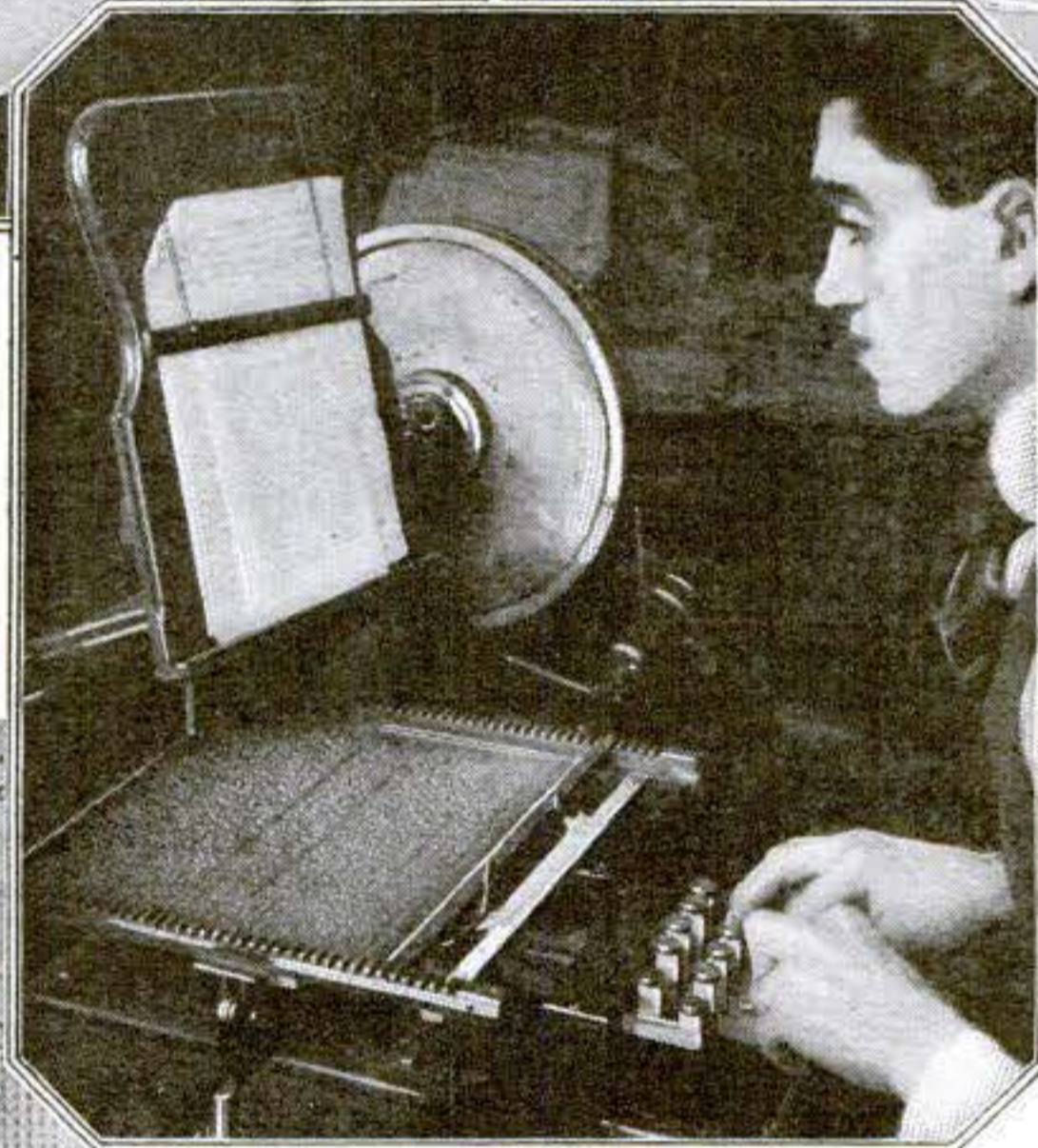
The dots of the Braille alphabet are punched into thin copper plates by a machine greatly resembling a typesetting machine. One of the plates serves as the stamp, the other as the die in the embossing. They register perfectly, being made by one operation
