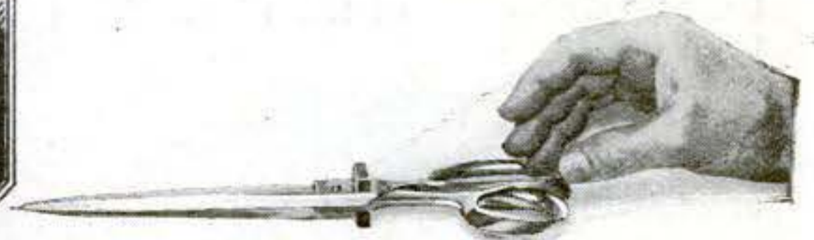
An attachment for keeping scissors in a convenient position for picking up
