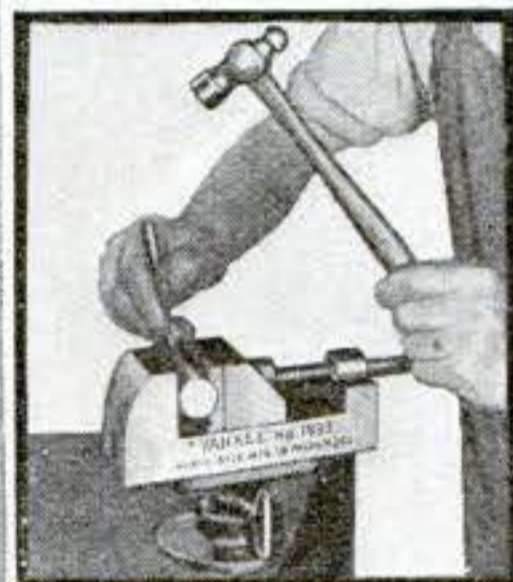
2. The centers on the cylinder as above marked, being punched for drilling.
