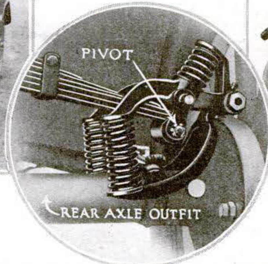
This shock-absorber for Fords has three coiled springs and four of them are used for each car
