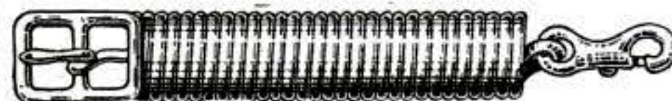
A compressed coil spring with buckle and snap to take the strain from the cloth
