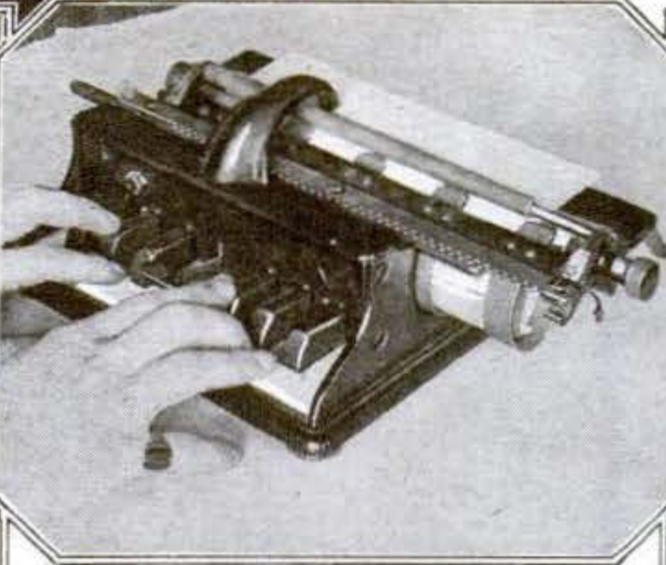
The typewriter for the blind has only six keys. Used in different combinations they emboss the desired characters of the alphabet in groups of raised dots on the paper. In this respect the mechanism of the machine very closely resembles that of the ordinary business typewriter
