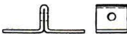
The metal bent to substitute an eye-bolt
