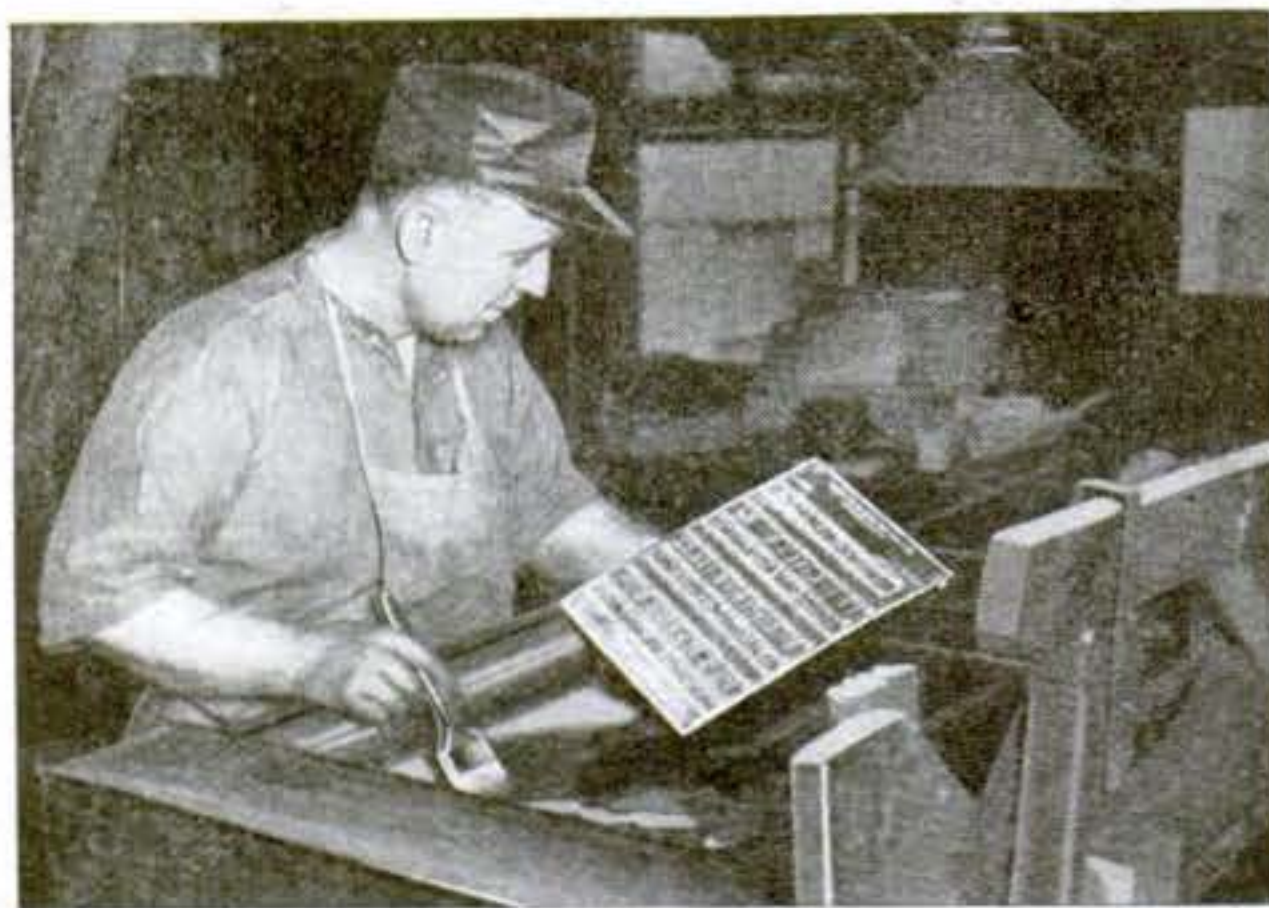
At this stage the plate from which notes and words are to be printed is etched in an acid bath
