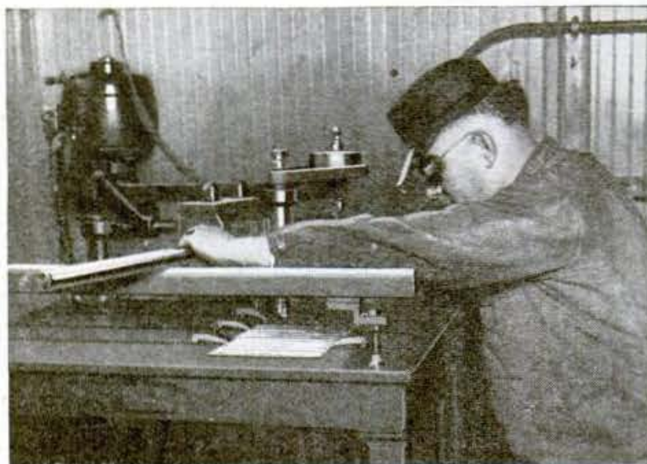
The "router" must carefully cut away the metal to make the notes and word type ready for printing
