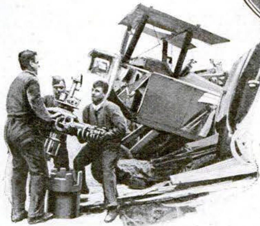
A single fast dive means taking apart the engine to clean out the soot
