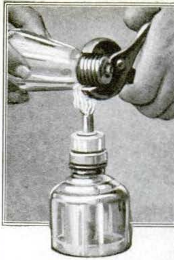
Removing the metal base from the globe without breaking the glass
