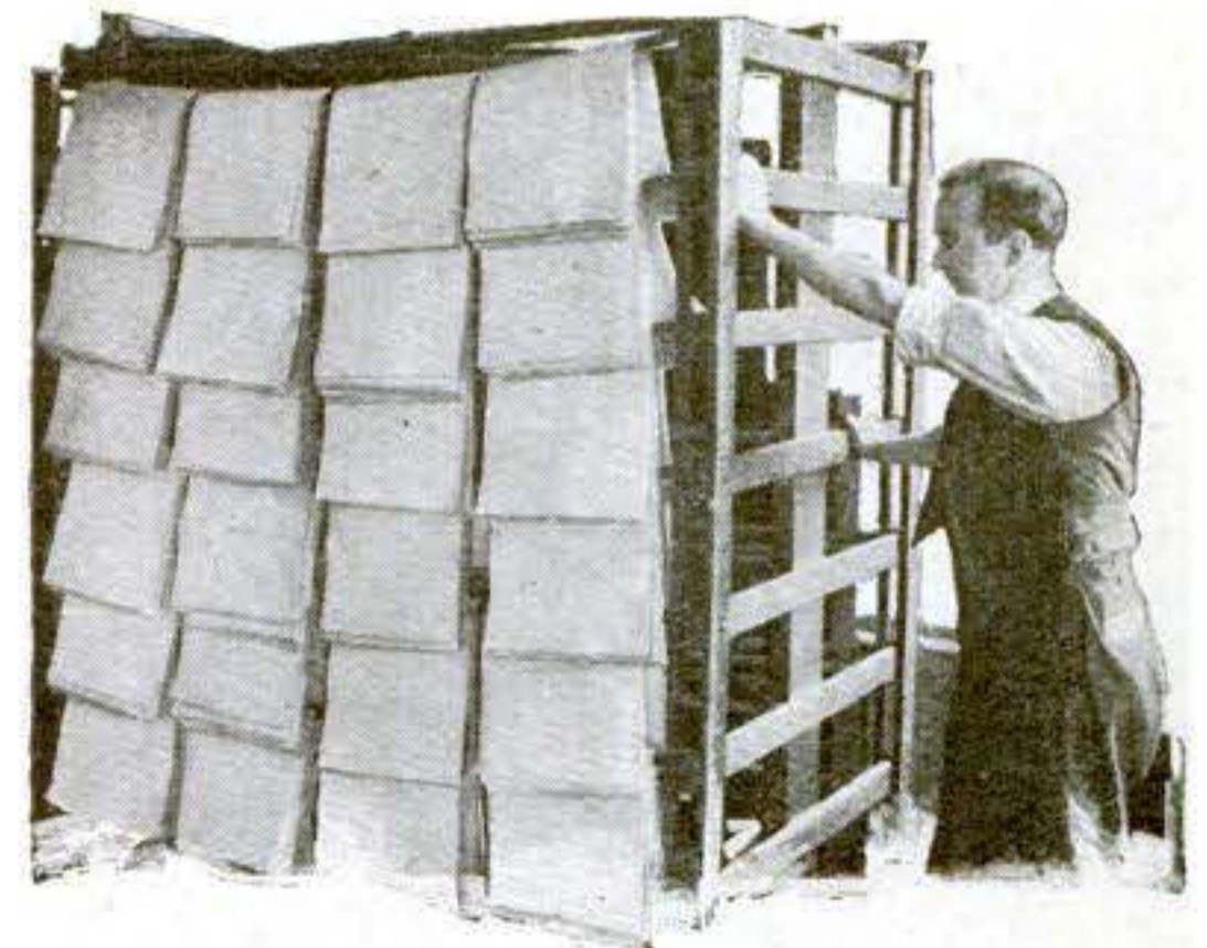
When the embossed sheets come from the printing-press they are still wet, and they are dried on racks before they are assembled in the final form
