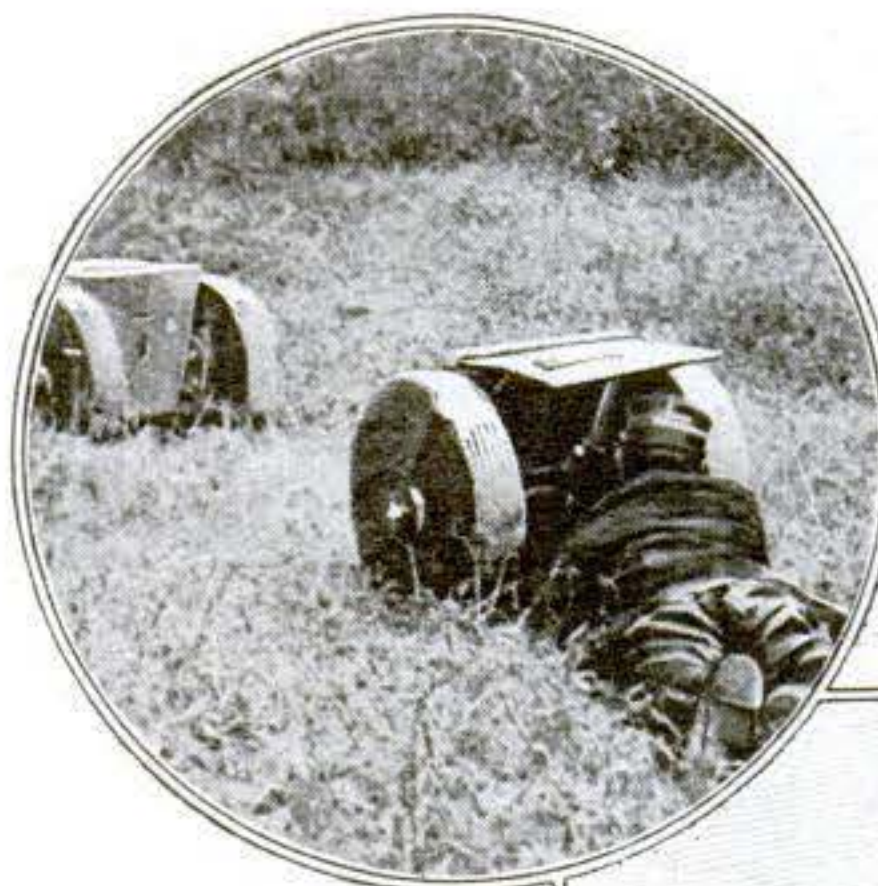
Protected by this shield against rifle and machine-gun bullets, they cut barbed-wire fences
